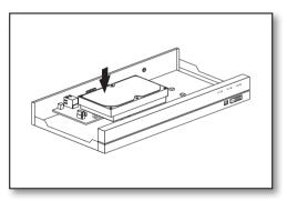
**4.** Multiple groups of screw mounting holes are provided on the bottom of the NVR. Screw the hard drive in place according to the size of your hard drive.
